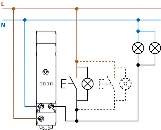
**Wiring diagrams** - 14.01 or 14.71 without Staircase maintenance function, triggered by PIR movement detector (18 series).
