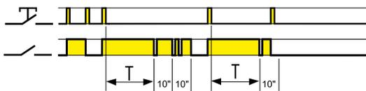
**(IP) Timing step relay with early warning**
