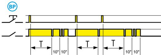
**(MP) Staircase timer with early warning + Staircase maintenance**
