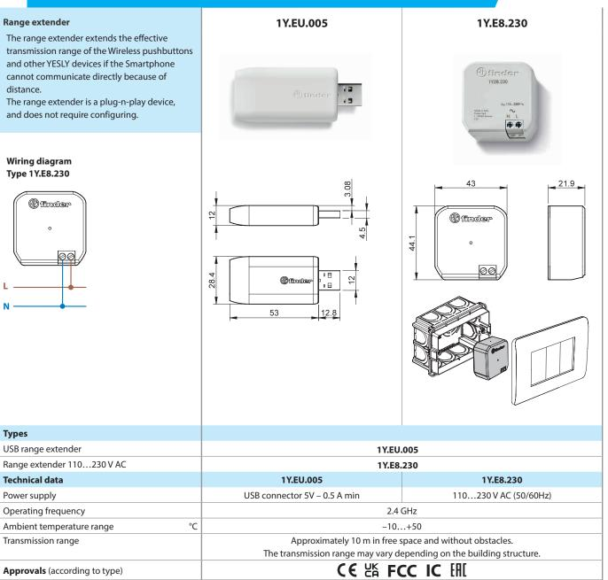
The range extenders must be installed within a maximum distance of 10 meters, and up to 4 devices can be used in the same system. It can be installed in any USB input that provides a power supply of at least 5V and 0.5A.
